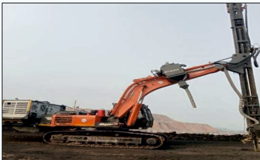
Drill Operation by Wet Drill Machines
