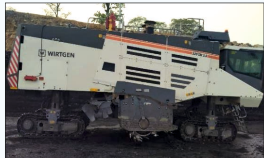
Coal Extraction through Surface Miner
